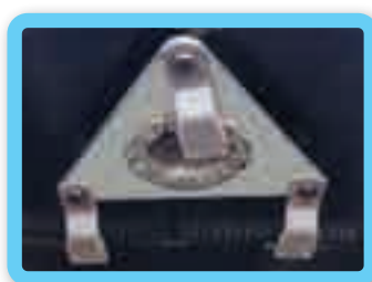
60" unit features three double-sided blades on a 3/4" thick blade carrier
