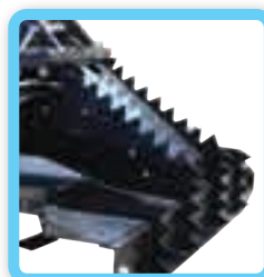
Serrated teeth to help move debris
