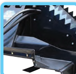
Removeable sides to access blades
