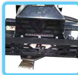
Open front exposes 2 1/4" of cutting blades
