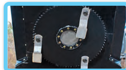
Three double-sided blades on a 1" thick blade carrier
