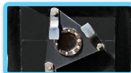
Three double-sided blades with a 1" thick blade carrier
