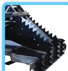
Serrated teeth to help move debris
