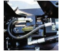
Hydraulic Piston Motor Adjustable Displacement Motor (45cc)
