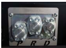
Centralized Hydraulic Ports and Greasing Points Easy Hookup and Maintenance
