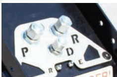
Centralized Hydraulic Ports and Greasing Points Easy Hookup and Maintenance
