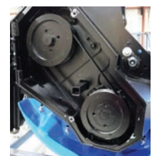
Synchronous Drive System Poly Carbon Fiber Drive Belt
