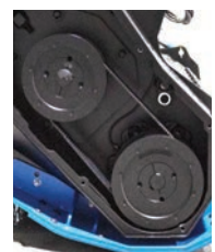
Synchronous Drive System Poly Carbon Fiber Drive Belt
