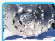
TEETH ON TOP, SIDE, AND BOTTOM OF CARRIER
