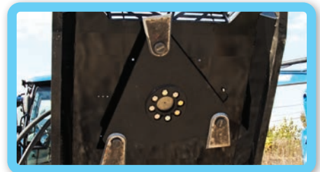
Three double-sided blades on a 3/4" thick blade carrier
