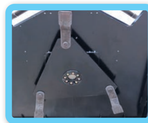
Three drop-down blades on 3/4" Steel Blade Carrier
