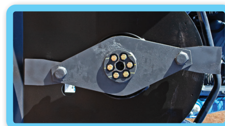
Two double-sided blades on a 5/8" thick blade carrier
