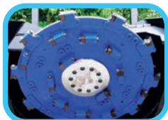
Teeth on top, side, & bottom of carrier
