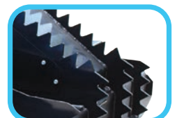
Serrated teeth to move debris
