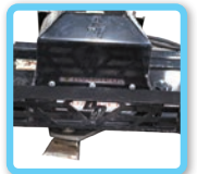
Open front exposes 2 1/4" of cutting blades
