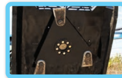
Three double-sided blades on a 3/4" thick blade carrier
