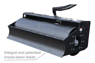
The Blue Diamond<sup>®</sup> Vibratory Roller has a patented exciter system with an advanced shaft design that reduces deflection by approximately 70% and reduces system heat by up to 100°. This significantly improves service life of bearings, seals and lubricants.
