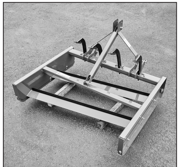
Figure 5: Dual Edge Grader blocked up on 4" x 4" wooden supports.
