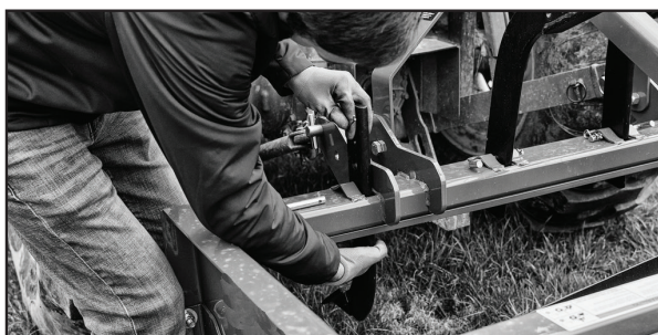
Figure 4: Place shank points down and forward to scarify.
