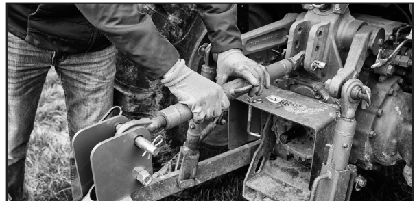
Figure 3: Use tractor top link to tilt front and rear of Dual Edge Grader.
