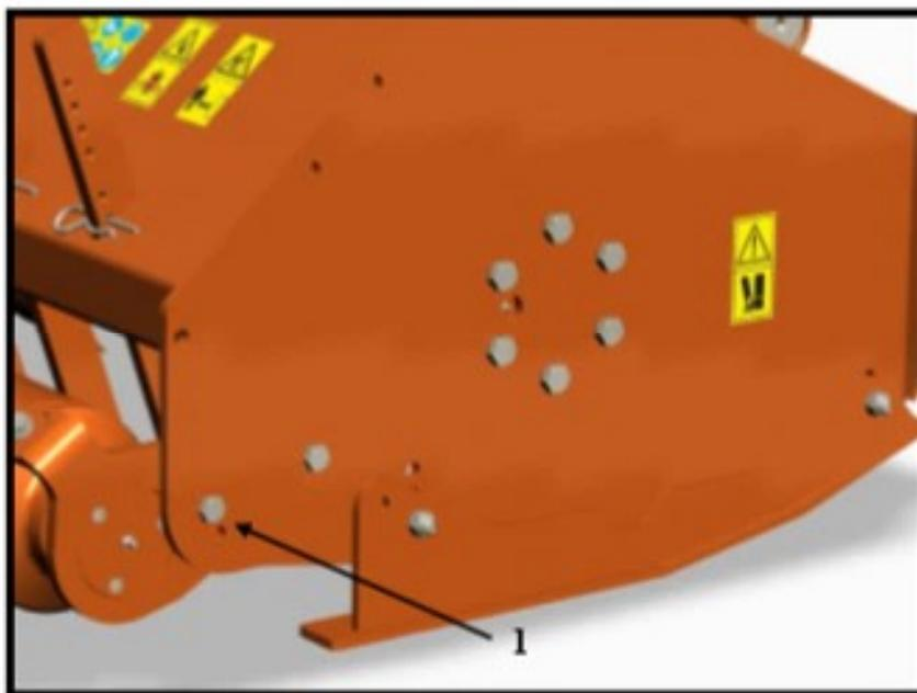
Depending on the different roller positions, it is possible to set four different cutting heights: 32-57-82 and 107 mm.
