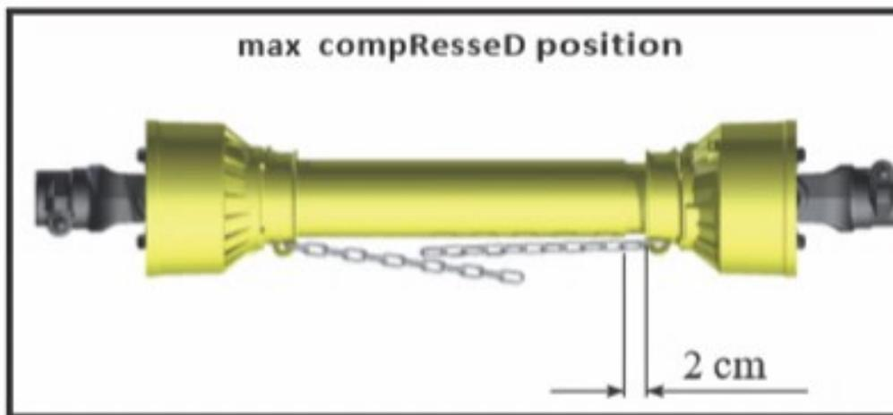
A driveshaft too long may cause structural damages to the tractor and machine. If the driveshaft is too long, it may be adapted by removing it and shortening the tubes according to the instructions provided by the Manufacturer in its use and maintenance manual.
