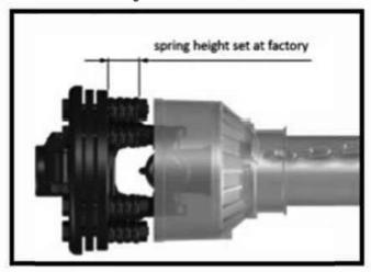
An adjustment can be done, however, when the dutch slipping is too frequent, which means that the calibration is too low.
