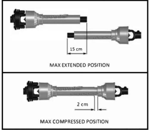
A driveshaft too long may cause structural damages to the tractor and machine. If the driveshaft is too long, it may be adapted by removing it and shortening the tubes according to the instructions provided by the manufacturer in its use and maintenance manual.
