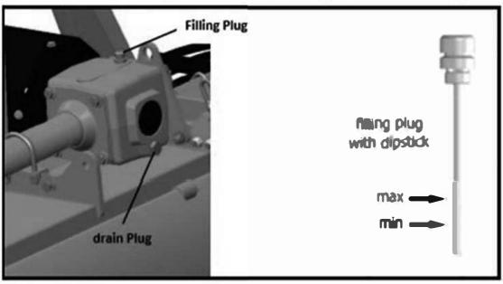
If the sign is below the minimum, fill up oil till restore the correct level.
