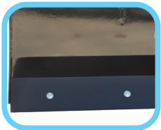
Two reversible and replaceable, curved cutting edges
