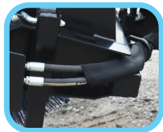
Hose routing to protect hoses
