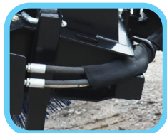
Hose routing to protect hoses
