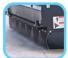
Pressurized water system
