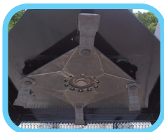
72" unit features four double-sided blades on a 3/4" blade carrier
