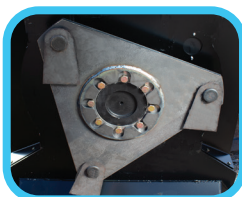
3 double-sided blades on a 3/4" thick blade carrier
