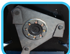
3 double-sided blades on a 3/4" thick blade carrier
