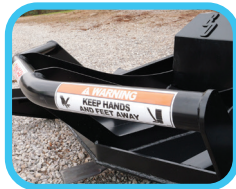
Heavy duty push bar for operator safety
