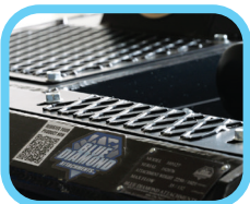
No slip tread for easier cab access
