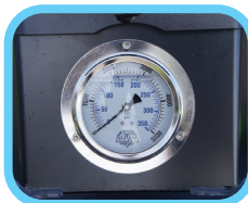
Pressure gauge helps prevent excessive stalling and overheating
