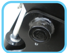
1 1/2" thick hinge pins and greaseable pivot points
