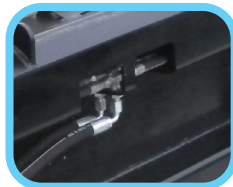
Hose routing protects hydraulic lines
