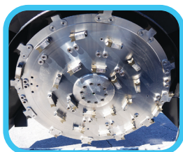
Teeth on top, side, and bottom of cutting disc
