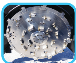
Teeth on top, side, and bottom of carrier blade
