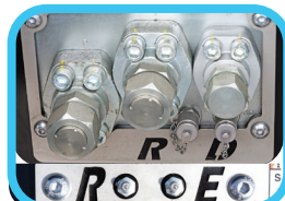
Labeled hose & grease ports
