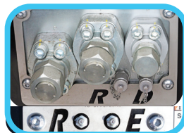
Labeled hose & grease ports
