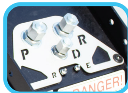
Labeled hose & grease ports
