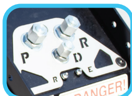
Labeled hose & grease ports
