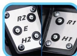
Centralized grease ports
