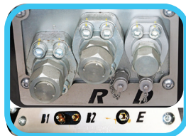
Labeled hose & grease ports
