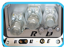
Labeled hose & grease ports
