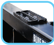
Safety steps on skid steer model for easy cab access
