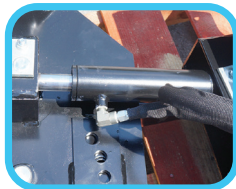
Hydraulic angle kit is optional. Blade tilts up to 10° and angle up to 30°
