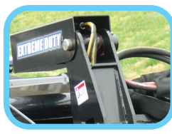
"No-pinch" hose routing
