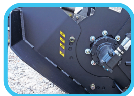
Adjustable foot keeps trench depth constant
