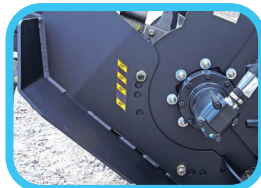
Adjustable foot keeps trench depth constant
