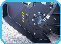
Adjustable foot keeps trench depth constant
