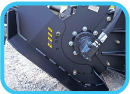
Adjustable skid foot keeps trench depth constant
